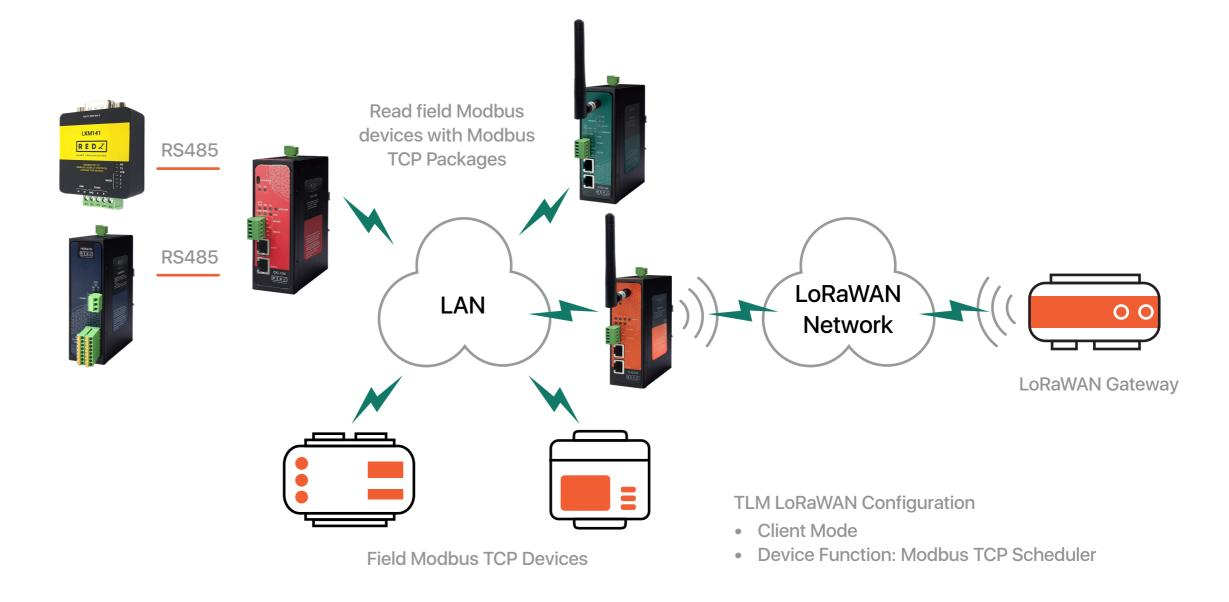
TLM Series LoRaWAN EndNode Modems can create a link between field devices and LoRaWAN server. Field devices with TCP/IP connectivity can be read via Modbus TCP protocol and data can be sent to LoRaWAN Server. Also field devices with RS232/RS485 Serial interface can be read in Modbus RTU protocol and data can be sent
