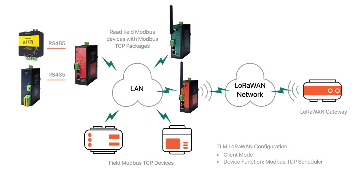
TLM Series LoRaWAN EndNode Modems can create a link between field devices and LoRaWAN server. Field devices with TCP/IP connectivity can be read via Modbus TCP protocol and data can be sent to LoRaWAN Server. Also field devices with RS232/RS485 Serial interface can be read in Modbus RTU protocol and data can be sent
